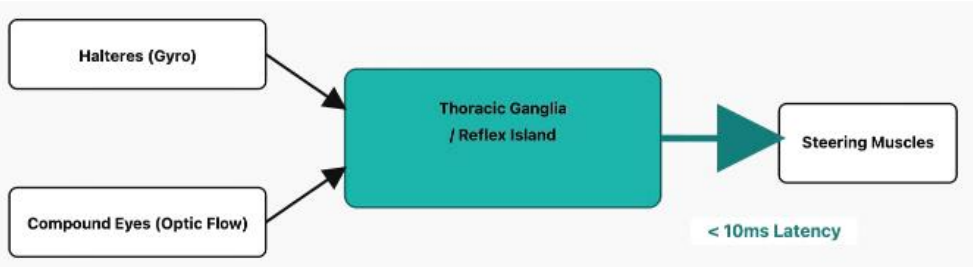
Figure 1.1: A schematic diagram illustrating the tight sensor-compute-actuation loop in Drosophila [1,2,3,4,5].
