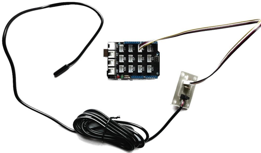
Figure 27: The body temperature sensor connected to the Arduino prototyping platform
